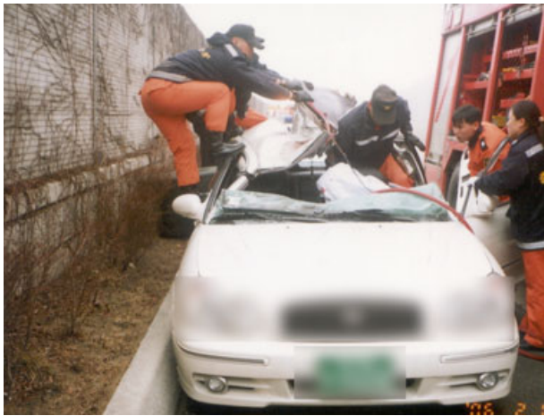
FIG. 3—The passenger car struck by failed wheel (refer to Fig. 2). Windshield and roofs are struck by the failed wheel.
