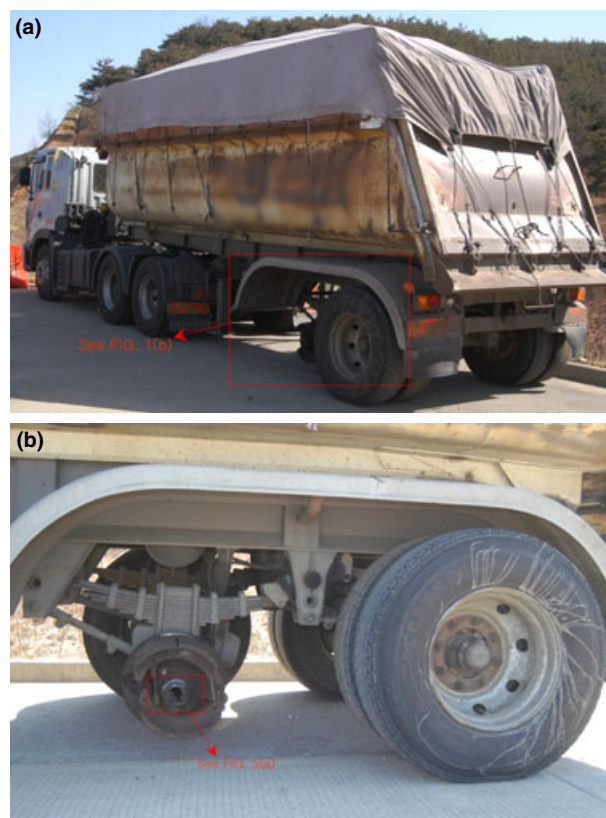
FIG. 1—The trailer with failed axle. The left first axle is completely fractured.
