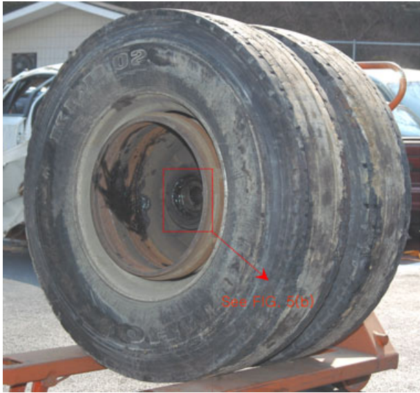
FIG. 2—The failed wheel. The wheel is completely separated from the trailer because of the fracture of axle. The fractured surface of the axle shown in the brake drum is magnified in Fig. 5(b).
